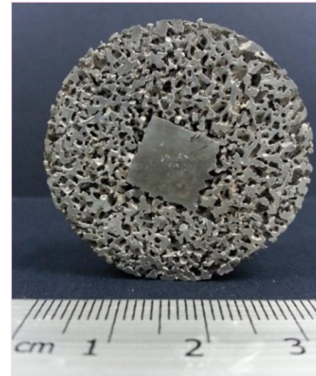
Aluminium foam with central pillar: (a) Top view (a) Side view
