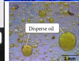
Fig 13. a) Collected product after HYSASE process, b) Oil droplet before gravimetric method (40x magnificant), c) Oil droplet after gravimetric method (470x magnificant), d) Oil droplet after gravimetric method with Black Sudan dye staining (470x magnificant).
